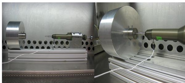
Figure 1: Impactor III device.
